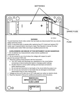
Figure 5-1. Battery and Fuse Compartment
