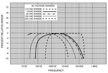
Figure 4-2. Typical Frequency Response, Output Ranges **18**
