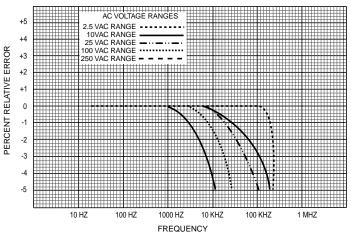
Figure 4-1. Typical Frequency Response, ACV Ranges
