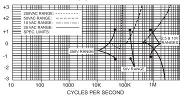
Figure 1-1. Typical Frequency Response Curve
