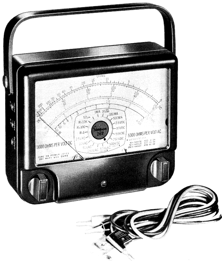
Fig. 1. Simpson Model 267 Volt-Ohm Milliammeter
