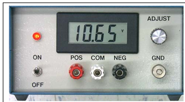
Figure 1.7 Front panel of power supply unit.
