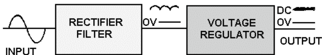
Figure 4-30.—Block diagram of a power supply and regulator.
